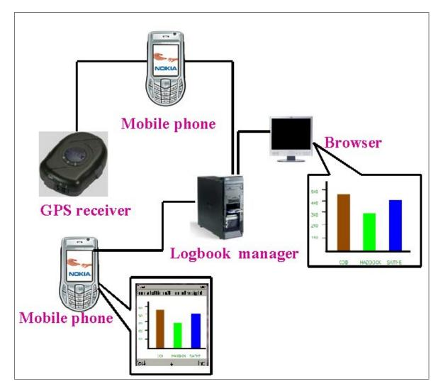
Figure 4.1: The system architecture for MLS.
