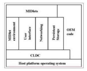
Figure 5.1: The Mobile Information Device Profile [32]
