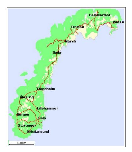
Figure 1.1: Telenor Mobil's GSM coverage.
