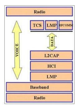
Figure 3.1: The Bluetooth protocol stack.
