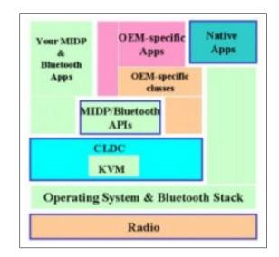
Figure 5.4: The architecture for J2ME CLDC/MIDP and Bluetooth.
