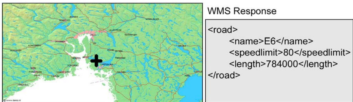
Figure 2.9: WMS GetFeatureInfo functionality
