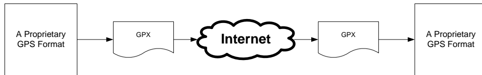
Figure 2.10: GPX used as a transport format
